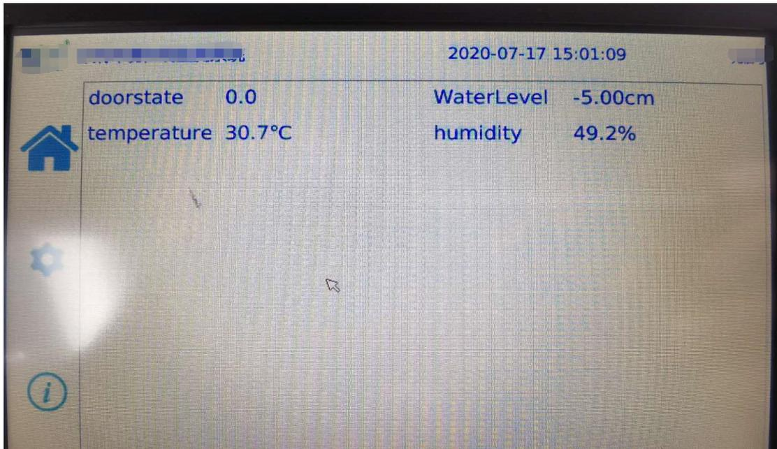
Note, TG462S LCD also provide change configuration via screen by press the Setting button, while the default password is “123456”
